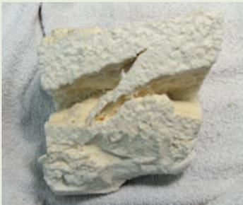
▲ Cracks, fissures, and voids in closed-cell foam indicate either a poor mix or excessive lift thickness.
