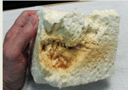
▲ Excessive exothermic heat can actually scorch foam, as shown here, and in extreme cases cause it to catch on fire.
