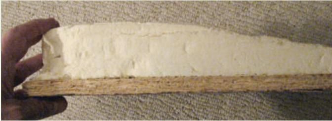
▲ Excessive moisture in the substrate can act as a blowing agent. Here, 2-pound SPF was sprayed on sheathing that was wet on the left side and dry on the right side. The foam on the wet side has increased in volume, compromising cell structure and substrate adhesion.
