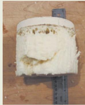
◀ The large void and delaminated area on this core sample indicate that the low-density foam was sprayed on a substrate that was too cold.
