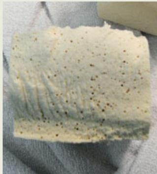
◀ High exothermic heat can also cause blowholes and discoloration in closed-cell foam.
