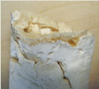
◀ In this example of off-ratio foam, the darkened layer at the top has very high compressive strength, an indication of an "A"-rich foam caused by a cold "B"-side component. Equipment malfunctions can also lead to off-ratio foam.
